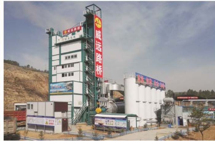
威远路桥4000H沥青混合料搅拌设备 4000H type asphalt mixing plant of the Weiyuan Road & Bridge company
