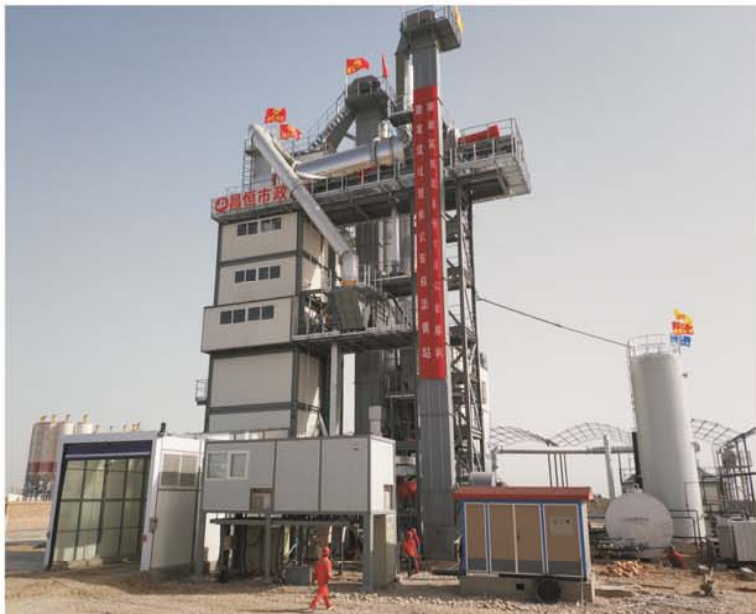
昌恒市政2000H型整体式沥青混合料再生设备 2000H type monolithic asphalt mixing recycling plant in municipal of Chang heng
