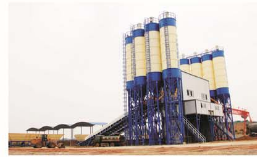
河南路桥2HZS90型水泥混凝土搅拌设备 2HZS90 type series Cement concrete mixing plant of Henan Road & Bridge Construction Group
