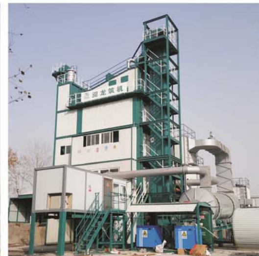
新郑公路局3000H型沥青混合料搅拌设备 3000H type environmental asphalt mixing plant of the Road Xinzheng City
