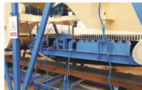
高精度电子秤 High-precision electronic scale
