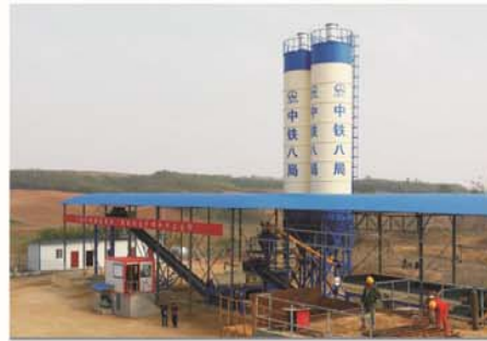
中铁八局WBC600型稳定土厂拌设备 WBC600 stabilized soil mixing plant China Railway No. 8 Engineering Group Co., Ltd.
