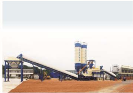
郑州港区JWBC800H型稳定土厂拌设备 WBC800 stabilized soil mixing plant of Air port, Zhengzhou city
