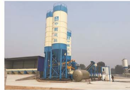
中建七局WBC1000H型稳定土厂拌设备 WBC600 stabilized soil mixing plant China Construction Seventh Engineering Division, Corp. LTD
