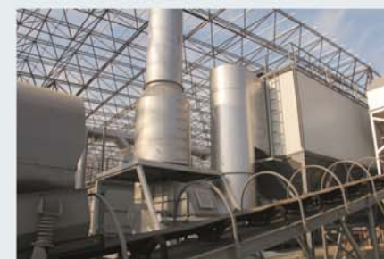
引风系统变频风机和消音器 Air induction system frequency conversion fan and silencer
