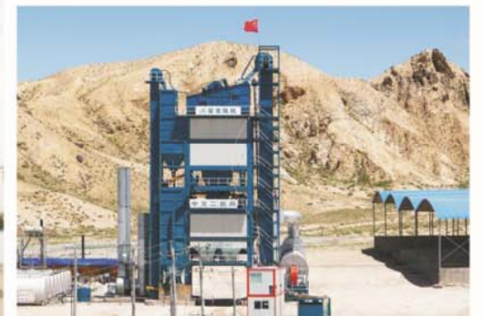
中交二航局4000型沥青混合料搅拌设备 4000 type asphalt mixing plant of the Second Harbor Engineering Company
