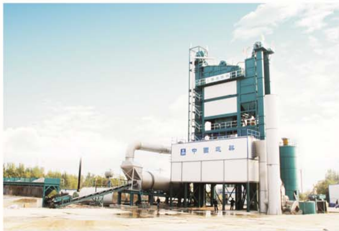
蒙新高速项目4000型沥青混合料搅拌设备 4000H type asphalt mixing plant of the mengxin high-speed project
