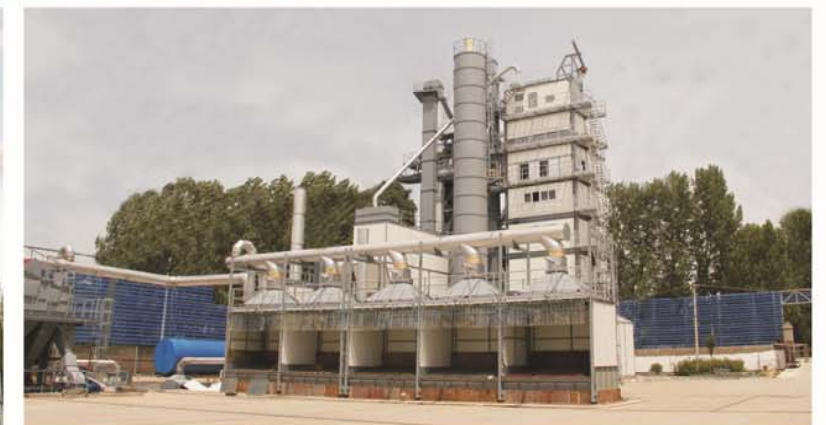
河南鑫龙路桥3000H型整体式沥青混合料再生设备 3000H type monolithic asphalt mixing recycling plant of the Xin dragon bridge company
