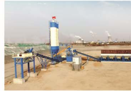
登封WBC600型稳定土厂拌设备 WBC600 stabilized soil mixing plant in Dengfeng city
