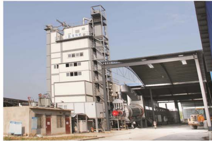
邓州市公路局4000H沥青混合料搅拌设备 4000H type asphalt mixing plant of Dengzhou highway bureau
