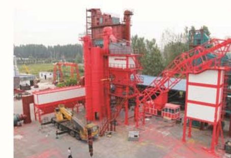
埃塞俄比亚1500型沥青混合料搅拌设备 1500 type asphalt mixing plant of Ethiopia
