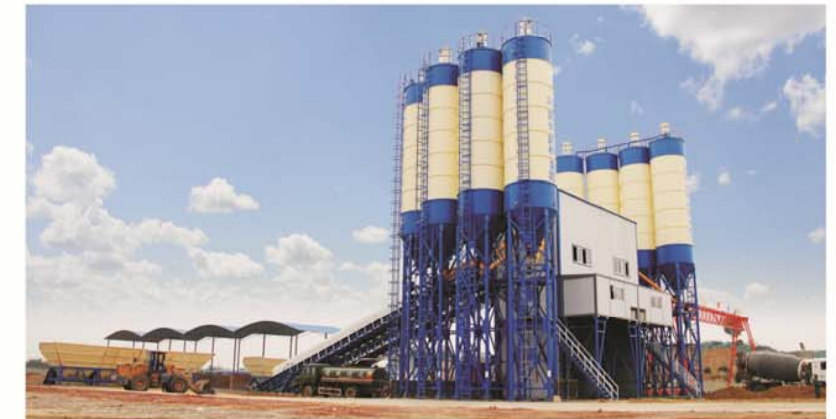
搅拌层计量层密封，负压集中收尘，零排放 The mixing layer and measurement layer are sealed; negative pressure collects dust, and realizes zero emissions;
