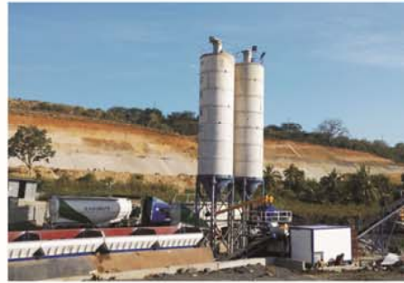
肯尼亚WBC600型稳定土厂拌设备 WBC600 stabilized soil mixing plant in Kenya
