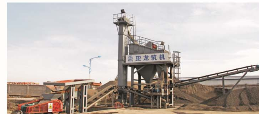
破碎筛分生产线，柔性破碎，高频筛分，避免回收料级配的二次破坏 Crushing and screening production line, flexible crushing, and high-frequency screening help prevent secondary damage to reclaimed materials grading.
