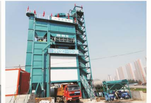
中交一公司4000型沥青混合料搅拌设备 4000 type asphalt mixing plant of CCC First Highway Engineering Co., Ltd.
