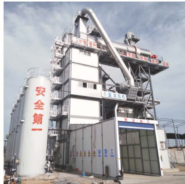
宁夏华晟3000H型整体式沥青混合料再生设备 3000H type monolithic asphalt mixing recycling plant of the HuaSheng company, Ningxia
