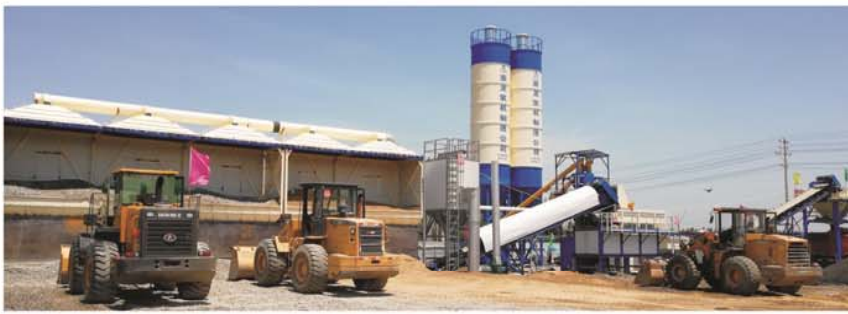
G207国道JWBC600H型稳定土厂拌设备 WBC600H stabilized soil mixing plant of G207 national highway
